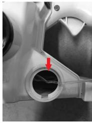
Replace the cap on the tank. Wipe any spillage if necessary.
